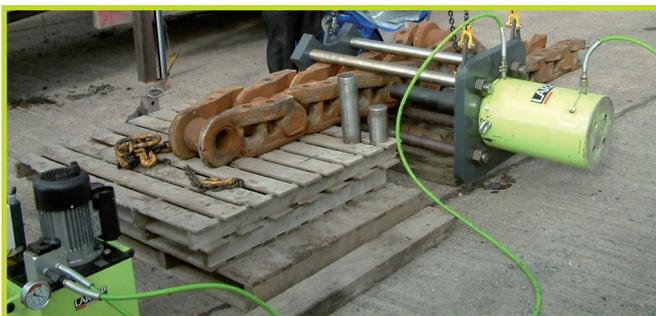
Double acting cylinders D35030, 350 ton and 300 mm stroke were used together with a HAM7645 110 volt 2.1 litre per minute power pack with remote control pendant for safety and ease operation.
