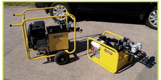
Petrol powerpacks for re-railing applications.
