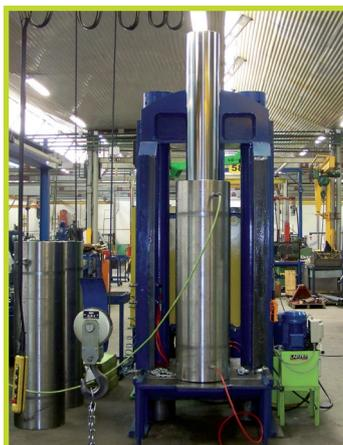
Double acting cylinder with 1.250 mm stroke.
