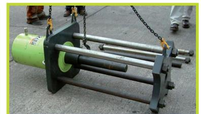
The pin was pushed through; in this case it took 251 metric tonnes to break the grip of the pin which was very badly worn.
