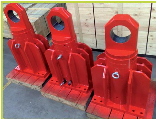
Double acting cylinders with lock nut and tilting saddle. Support a 10% side load.
