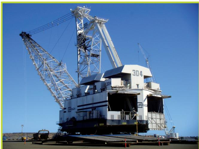
Larzep supplied the seven 500 Tn lifting cylinders for the tub lift-and-split, twenty two 100 Tn cylinders along with an electric power pack incorporating valving controlled electronically via a PLC, all controlled by the laptop for work on the 6400 Tn Marion dragline.
