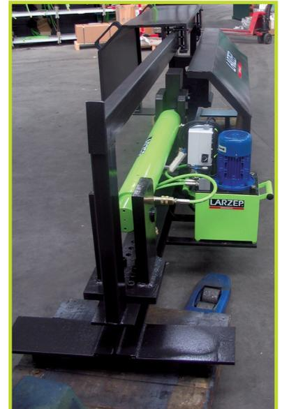
Wheel crusher. 23Tn capacity and 800 mm stroke.
