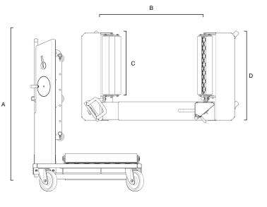
Side-adjustable lifting arms for wheel diameters ranging 1000-2400 mm (39.97 ÷ 94.48 in). Robust safety wheel retaining bracket for the safe manoeuvring of the trolley. Precise and easy mechanical lifting and lowering. Excellent manoeuvrability due to the 4 large, heavy-duty revolving wheels. Lifting arms fitted with 3 roller bearings for ensuring the easy location of the wheels.
