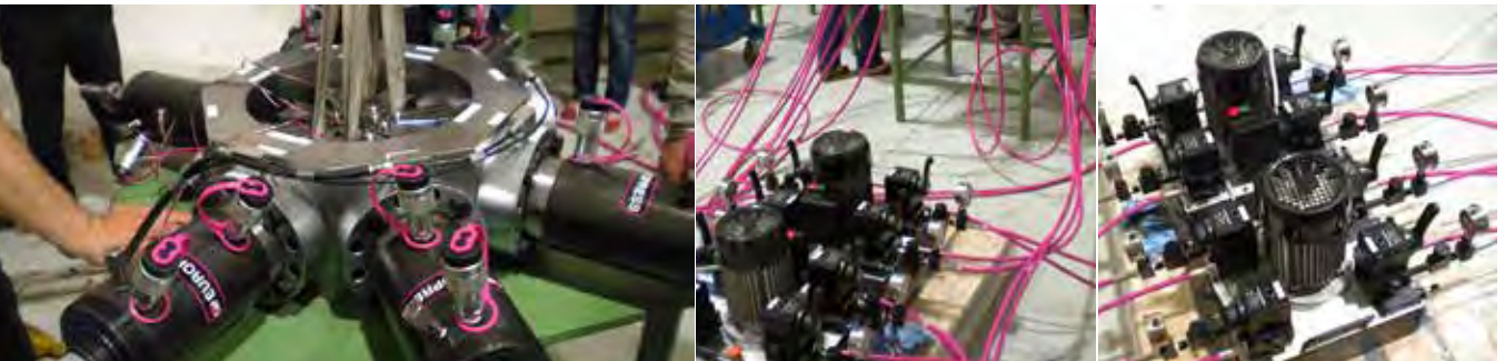
Crimping equipment for the hoses of a nuclear power plant. China.
