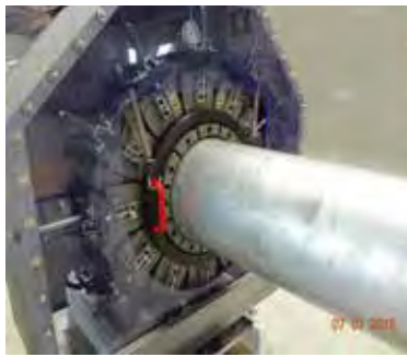
Combination of machineries for the crimping and expansion of aluminum hoses during crimping.
