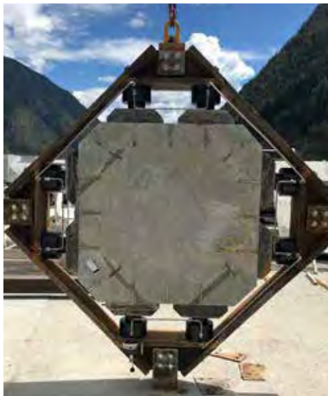
Special cylinders for high temperatures, fitted on resistance verification equipment to test flameproof concrete tunnel segments
