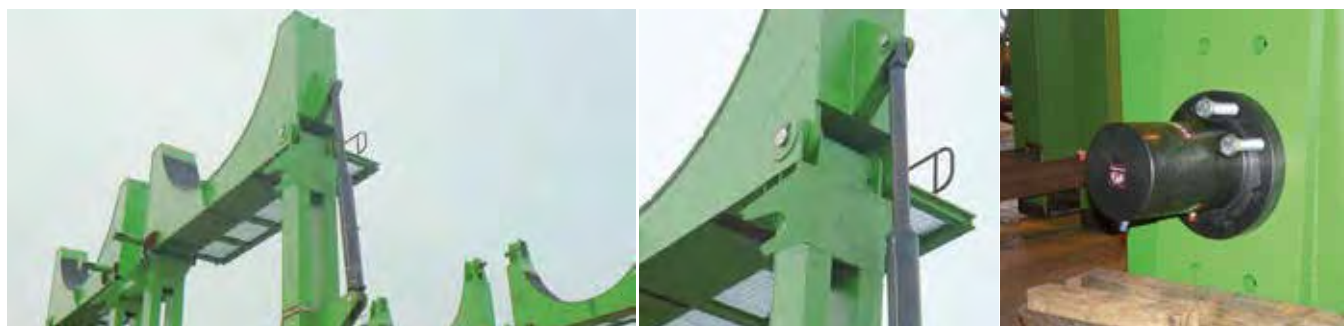
Long stroke cylinders useful for the operation of a mechanical arm for the installation of offshore wind turbine towers. U.K.
