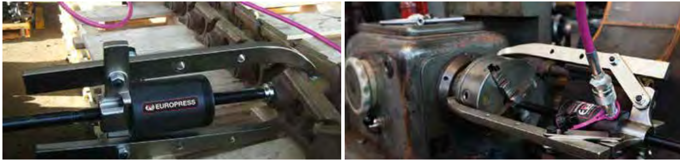
Quality testing of chains for tracks - Spindle extraction during the maintenance of the lathe.
