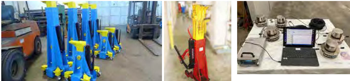
Monitoring system for loads on bearing points of a bridge.
