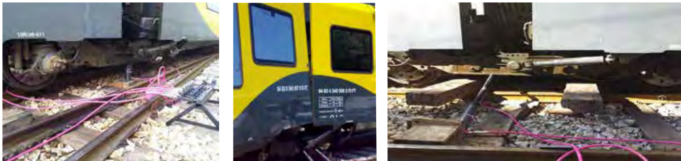
Example of telescopic cylinders, EPP valves and power packs for operations such as inspections, installations, and maintenances of railway infrastructures and vehicles.
