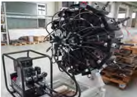
Combination of machineries for the crimping and expansion of aluminum hoses during crimping.
