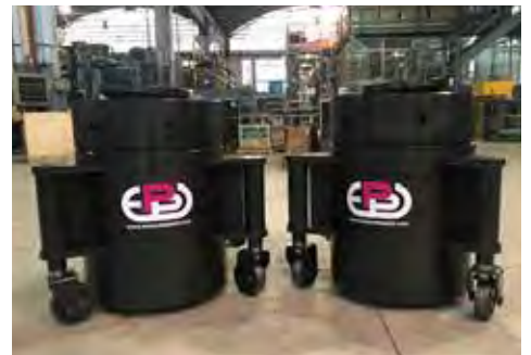
High tonnage cylinders with wheels for applications where mobility is important.
