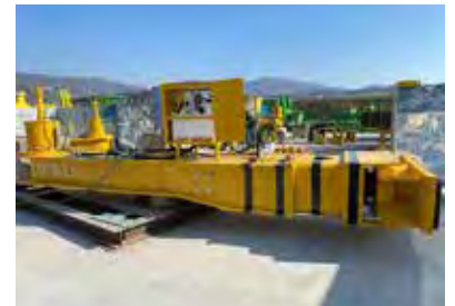
Stabilization systems for wind turbines' foundations with special cylinders and power packs suitable for marine environment.
