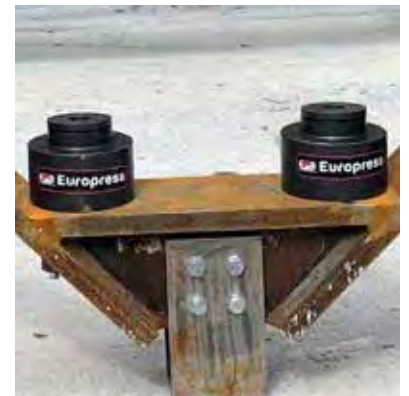
Special cylinders for high temperatures, fitted on resistance verification equipment to test flameproof concrete tunnel segments
